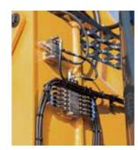
With the optional **auto greasing system**, grease is applied to lubrication points automatically when needed. The correct dosing is ensured and lubricant is applied uniformly, reducing grease consumption and eliminating waste.
