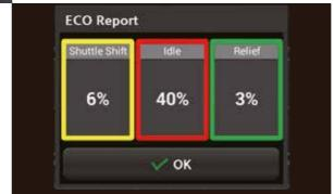
The **Eco Report** feature makes it easy for operators to develop efficient working habits by displaying real-time information about machine performance.
