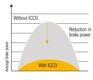
The Intelligent Clutch Cut-Off (ICCO) function minimises loss of power in the torque converter and prevents excessive power use during braking. This reduces heat generation and wear on the brake disc.
