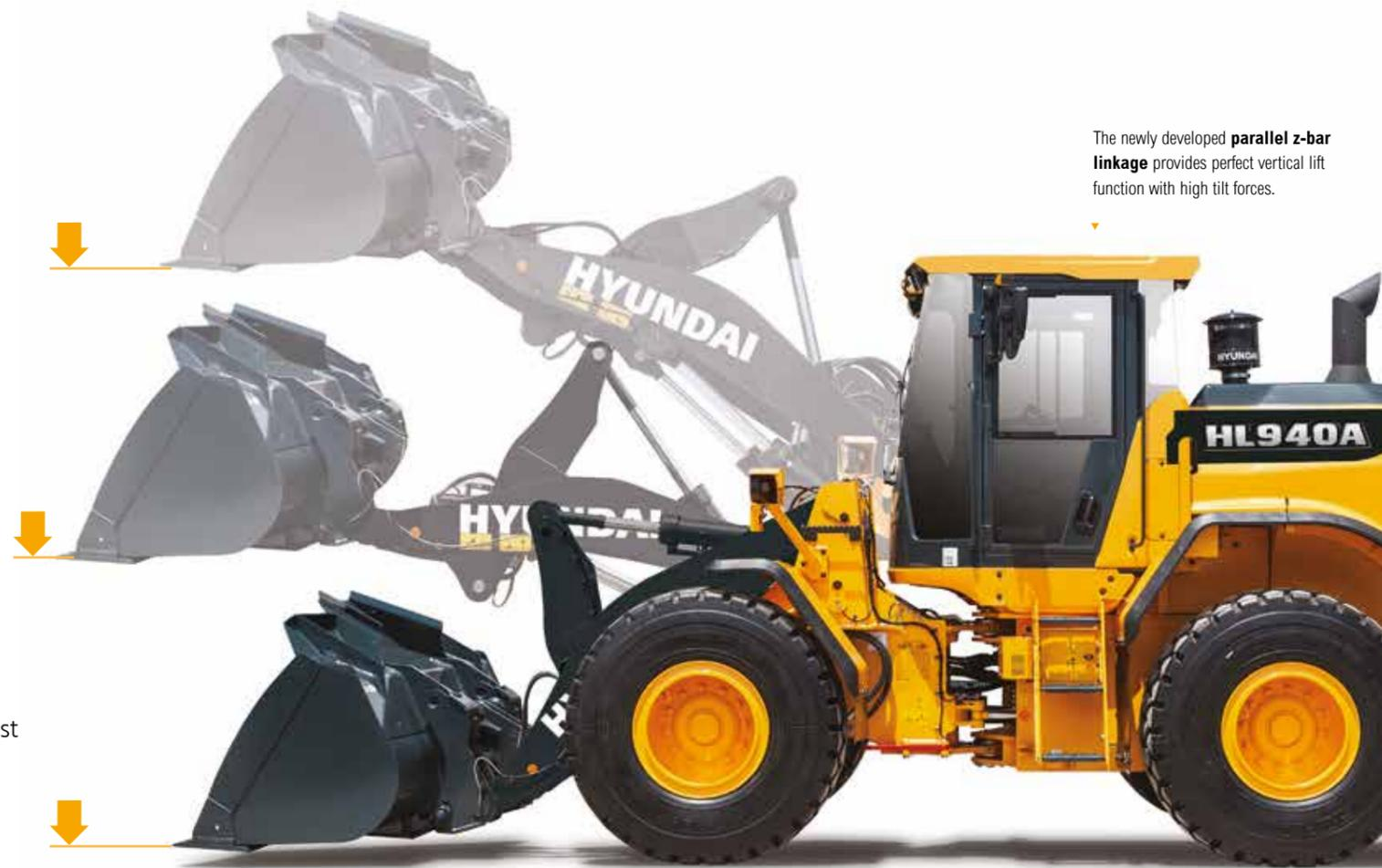
The newly developed **parallel z-bar linkage** provides perfect vertical lift function with high tilt forces.
