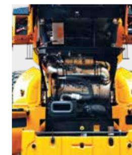
The **tilt-back engine hood is fully retractable** and can be **opened electrically** for easy access to the sealed engine room and cooling room. The engine room is designed to prevent the possibility of fire caused by the inflow of foreign materials.
