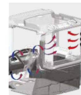
The **air conditioning system** is installed on the right side of the cabin for convenient maintenance and filter replacement. It features a high-capacity inner filter and a specially-selected filter material for superior performance.
